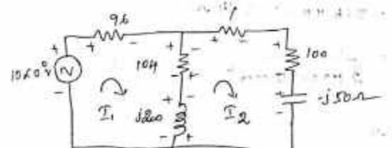
Step 2: Applying KVL to the two loops,
