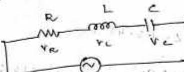
$$\begin{aligned} \therefore Z &= R + jX_L - jX_C \\ &= R + j(CL - \frac{1}{fC}) \end{aligned}$$
