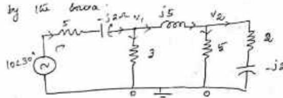
$$\frac{20 \angle 30^\circ - V_1}{5-j2} = \frac{V_1}{3} + \frac{V_1 - V_2}{j5}$$
